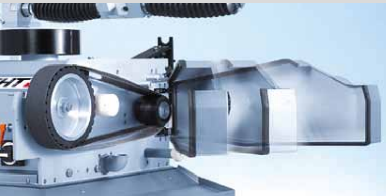
Grinding belt replacement
