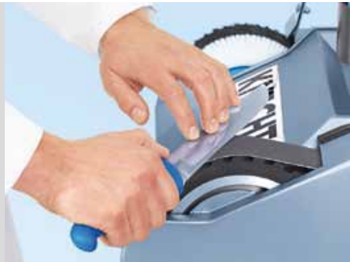
Sharpening hand knives on the wet-grinding belt
