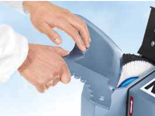
Polishing bowl cutter blades with the finned brush
