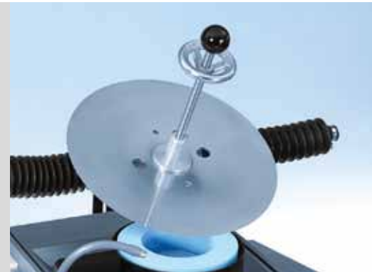
Circular blades (diameter 80-480 mm) sharpened with the cup grinding wheel
